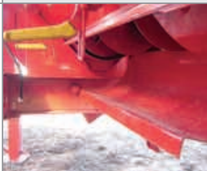
As an optional, a system of fast & uncoupling (Registered Trade Mark OMBU ) is provided to the base of the horizontal auger. This system prevents water and waste stagnation and makes the cleaning of the grain cart easier when different kinds of grains have been transported. Essential in harvesting for seeding plants. (Seeds basket)
