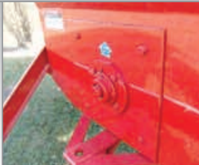
Rear Coupling and removable lid of the horizontal auger.
